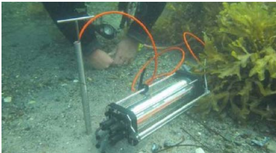
Fig. 23: The spear-like sediment profiler tested at Tudse Hage.
