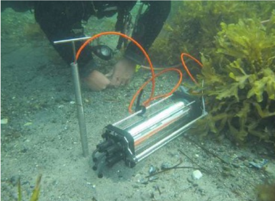
Fig. 10: The diver-operated datalogger with spear sediment profiler.
