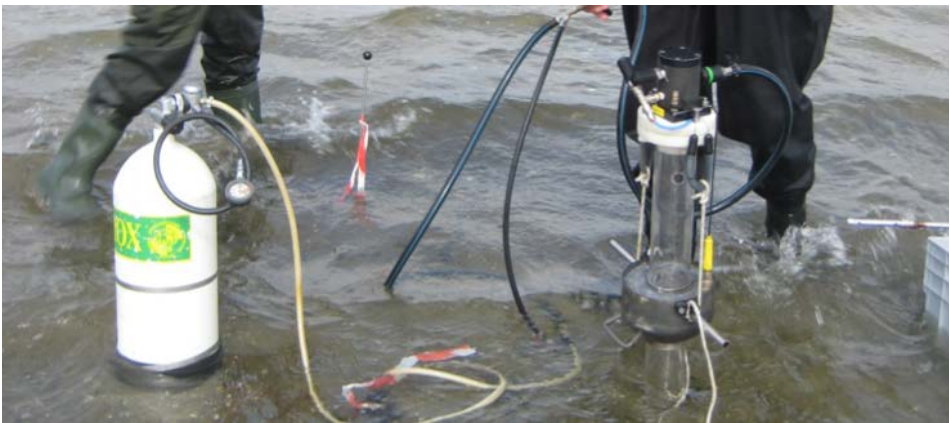
Fig. 25: Characterising the site environment ex situ by taking cores with the vibrocorer that has been developed within the SASMAP project
