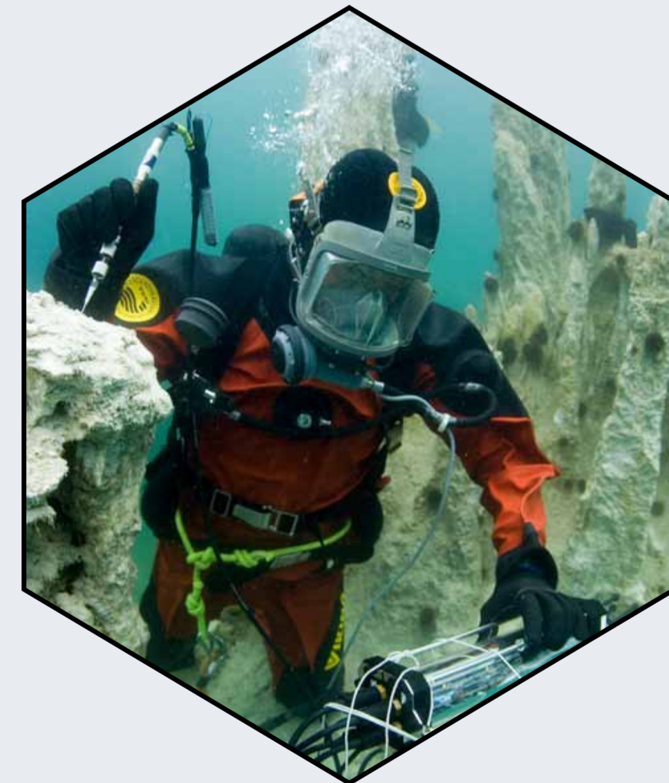
Diver using a micro sensor to measure environmental parameters underwater. Image: Unisense
